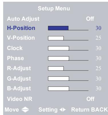
**Auto Adjust** - Automatically adjusts to the best image position, as well as the best clock and phase settings.
