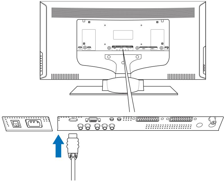
**NOTE:** To connect a DVI device, use a DVI-to-HDMI adaptor. You will also have to connect the audio cable from your DVI device to the PC Audio In connector.
