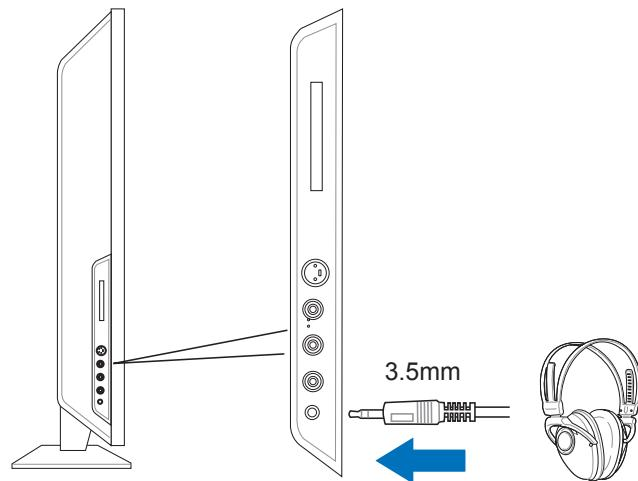
**NOTE:** When a headphone is connected, the TV's internal speakers are turned OFF.
