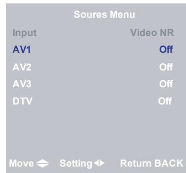
Set the Video NR for each input source from this menu. Turn Video NR ON to reduce on-screen noise.
