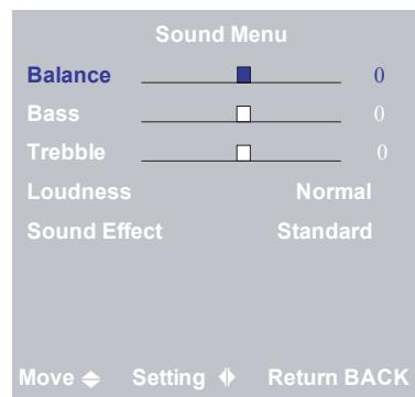
**Balance** - Adjusts the level of sounds between the left and right speakers.
