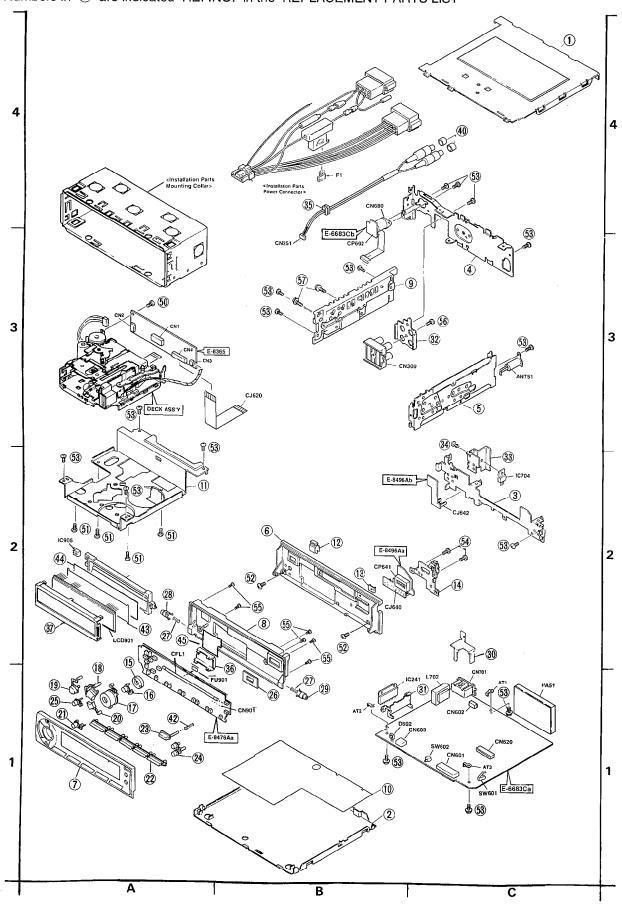
**EXPLODED VIEW (Tape Deck)**■ Numbers in ○ are indicated REF.NO. in the REPLACEMENT PARTS LIST
