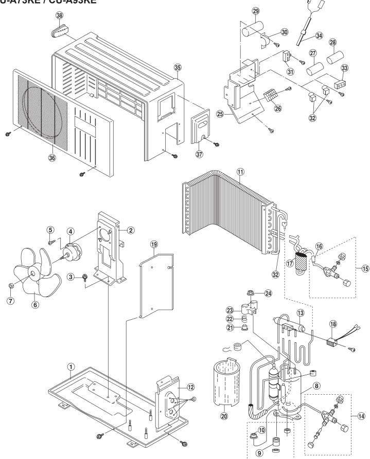
(Note) : The above exploded view is for the purpose of parts disassembly and replacement. The non-numbered parts are not kept as standard service parts.
