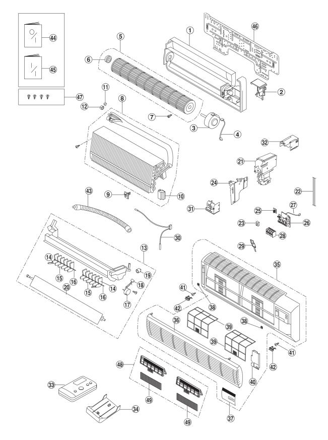
(Note) : The above exploded view is for the purpose of parts disassembly and replacement. The non-numbered parts are not kept as standard service parts.
