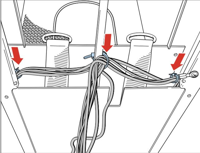
Disassemble MOVING COLUMN ASSY 15
