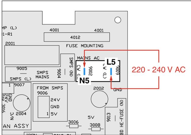
4.2 Check for output of 24 V DC and 5 V DC from switch mode power supply.
