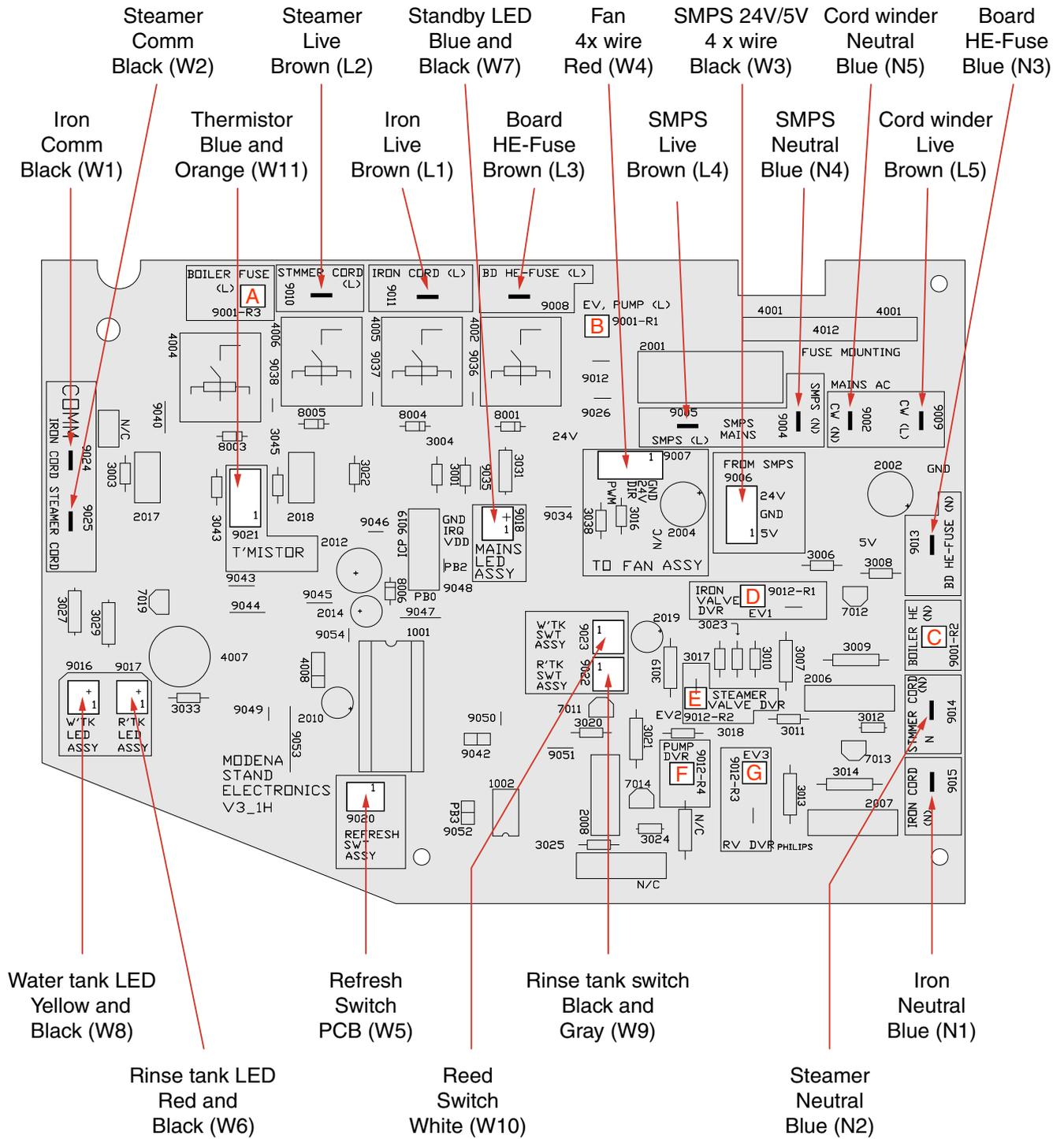
NOTE : ABC (brown, red, and blue) is a 3 pole connector to connect to boiler side. (W12)
