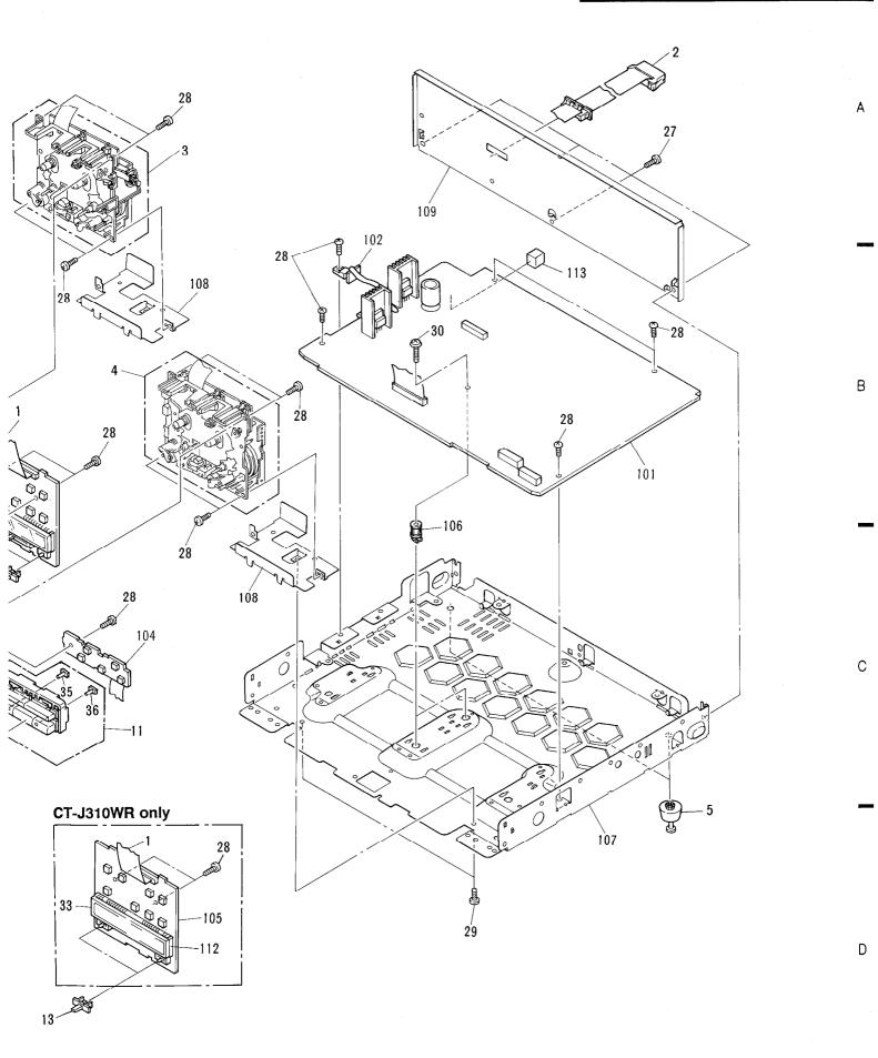
1.2 MECHANISM UNIT 1 (RYM1191): CT-J410WR and CT-J310WR
