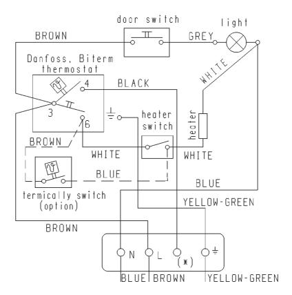
Connector \* is in the junction box market depending on producer of compressor as follows
