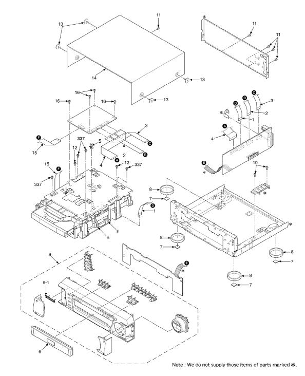
22. Loading Mechanism Parts Location
